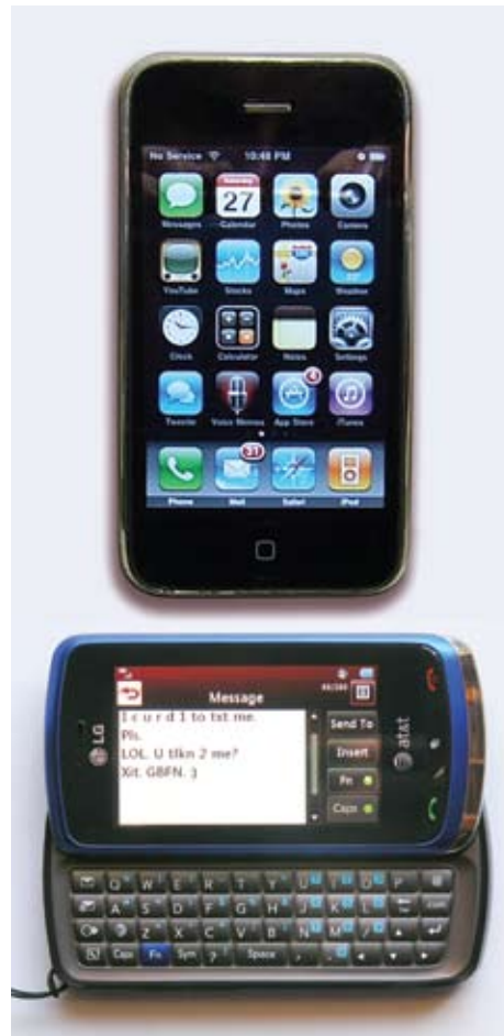
The iPhone (top) is an example of a device supporting SMS services via a touch screen. The LG phone (bottom) features a QWERTY keyboard to facilitate texting plus touch screen capabilities.
